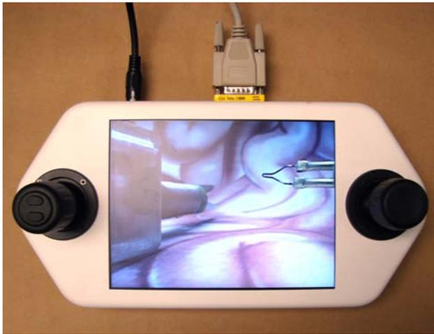
**Fig. 4** Surgeon console used for control of the natural orifice transluminal endoscopic surgery (NOTES) robot
