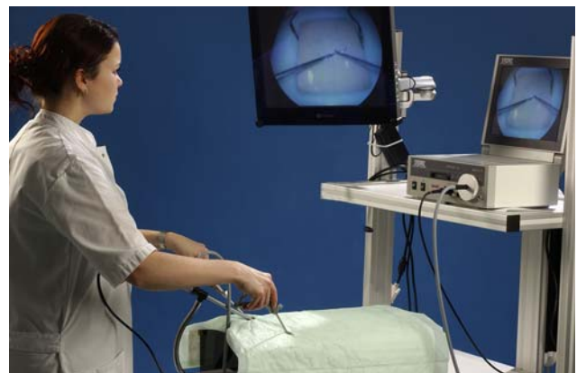
Fig. 1 Traditional box trainer, containing a foam suturing pad (Limbs & Things Limited, Bristol, United Kingdom), a Telepac system with endoscope (Karl-Storz Endoscope, Tuttlingen, Germany), video monitor (Neovo X17a), and needle holders (Karl-Storz Tuttlingen, Germany)
