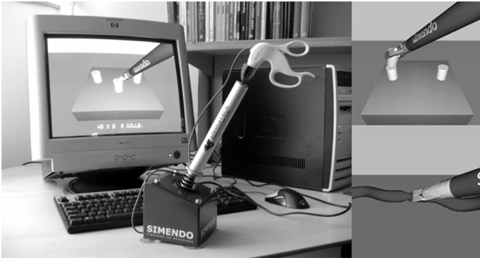
Fig. 1. Left: the SIMENDO connected to the PC via USB-port. Right: examples of exercises. Piling up of cylinders and clipping of a vessel.
