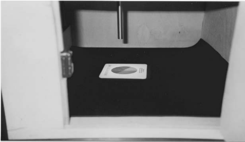
Fig. 2. Resolution card placed on black neoprene to reduce glare. The distance between the telescope and the paper was 100 mm.
