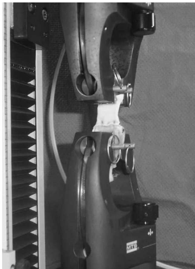
Fig. 8. Fixation strength testing of mesh/abdominal wall sample using an Instron MN44 tensiometer.
