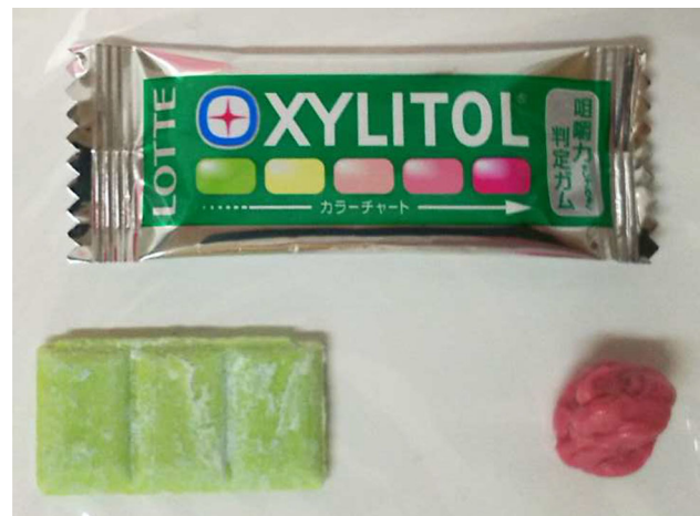
Fig. 1 The color-changeable chewing gum ( 70 \times 20 \times 1 \text{ mm}^3 ; 3.0 g). The gum changes color from yellowish-green (right side) to red (left side) after chewing. The red dye is pH-sensitive and changes color under neutral or alkaline conditions. Citric acid maintains a low internal pH of the yellowish-green gum before chewing. As chewing progresses, the gum changes to red because the yellow and blue dyes seep into the saliva and the red color appears as a result of citric acid elution. Changes in the color values of the gum reflect the comprehensive ability of mastication
