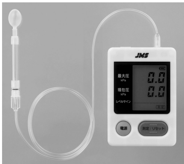
Fig. 1 Maximum tongue pressure measurement instrument (JMS, Hiroshima, Japan)
