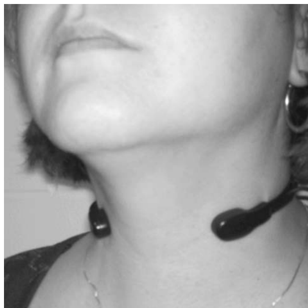
Fig. 1 This image shows the location of the microphone used in the natural-drinking task to acquire an audio recording to assist in identifying the location of sip-swallow events. The receiving heads of the microphone were positioned over the lateral aspect of the larynx, just inferior to the thyroid cartilage, and equidistant from the midline
