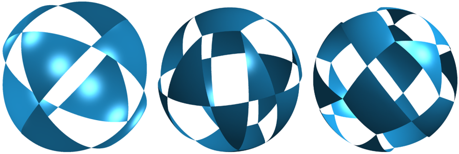
Fig. 6 Examples of partitions of the sphere containing spherical parts of Meissner or Reuleaux polyhedra and spherical rectangles
