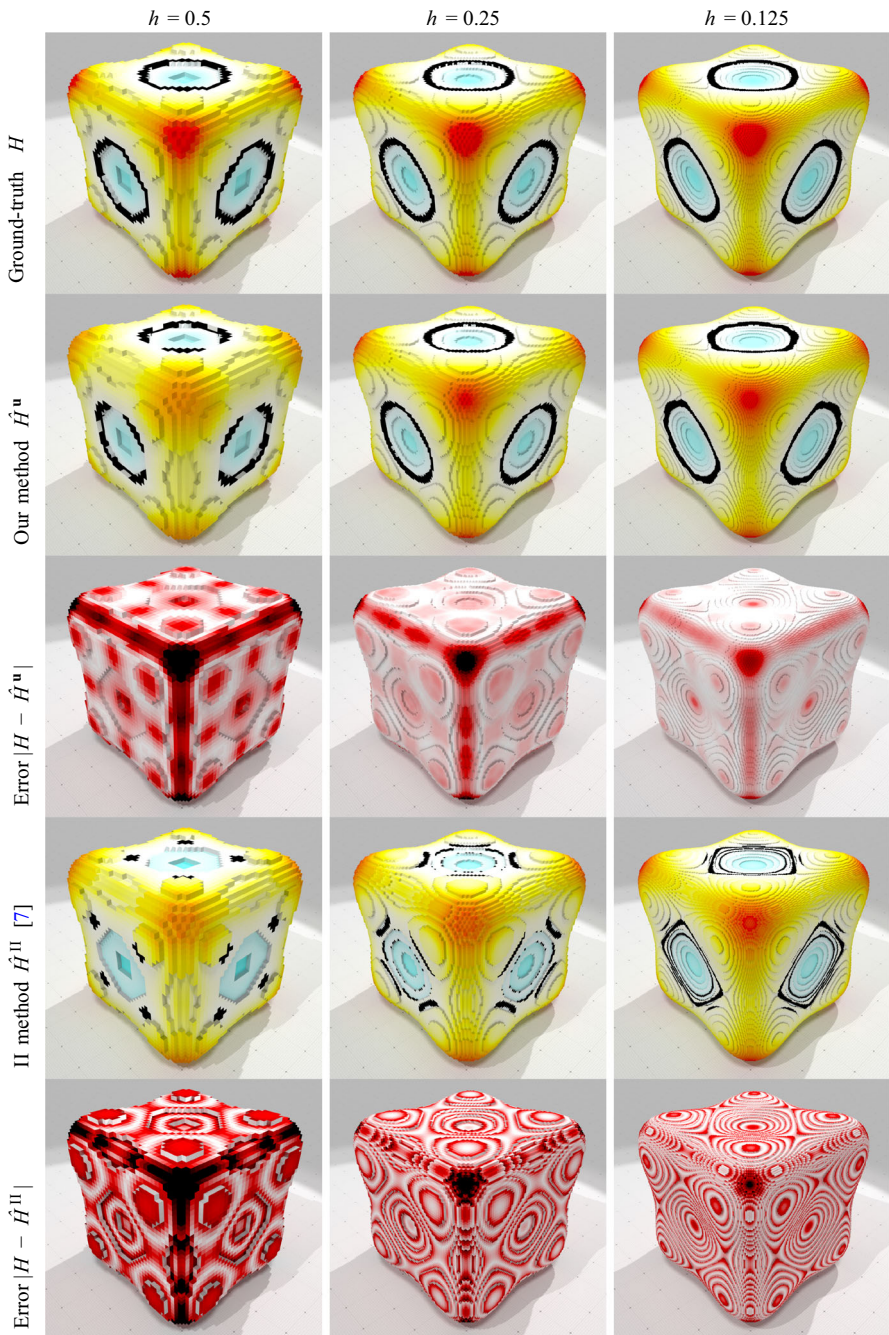
Fig. 9 Illustration of the accuracy of mean curvature estimators \hat{H}^u and \hat{H}^{II} at different resolutions: 1st row is ground-truth H , 2nd row is our approach \hat{H}^u , 3rd row is its local estimation error |\hat{H}^u - H| , 4th row is integral invariant approach \hat{H}^{II} , 5th row is its local estimation error |\hat{H}^{II} - H| . Curvatures are displayed with colors from dark blue ( -0.3 ) to white to red ( 0.3 ), except a black band at [-0.01; 0.01] . Errors are displayed with colors from white ( 0 ) to red ( 0.025 ) to black ( 0.05 )
