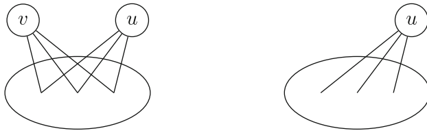
Fig. 3 a The graph G that has a twin \{u, v\} ; b the graph G' after deleting v from G and updating the weight of u by letting w(u) = w(u) + w(v)
