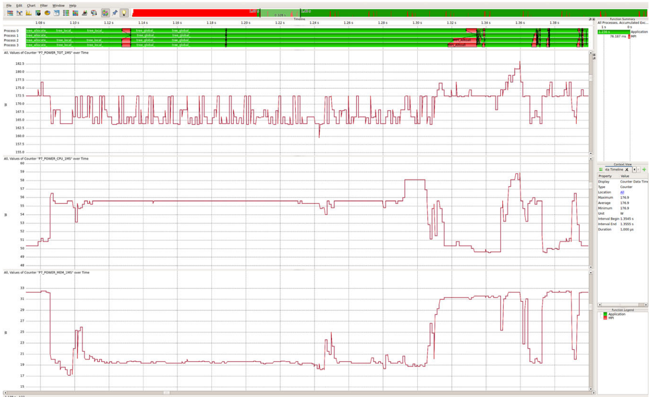
Fig. 5 Vampir screenshot of one iteration of a PEPC run showing that there are significant changes in power consumption at millisecond scale
