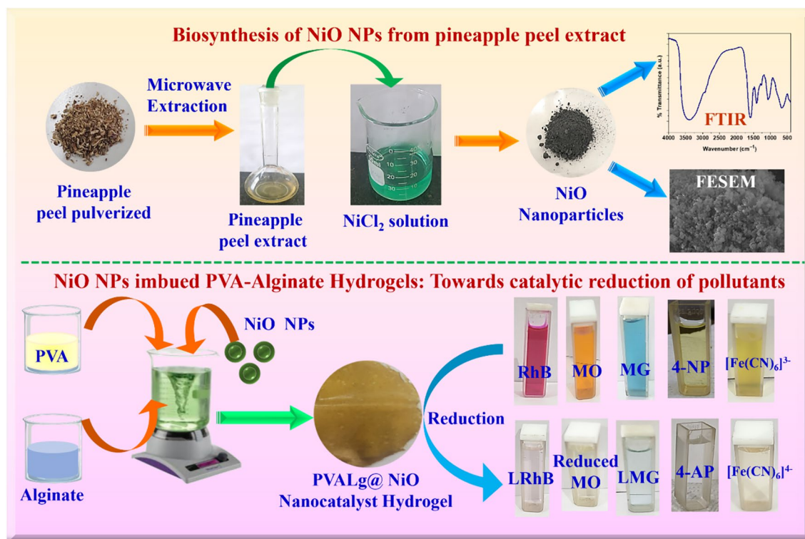
Scheme 1 Schematic depiction of biosynthesis of NiO nanoparticles from pineapple peel extract. The nano NiO was integrated into PVA–alginate hydrogels to form nanocomposite hydrogel (PVALg@ NiO).
