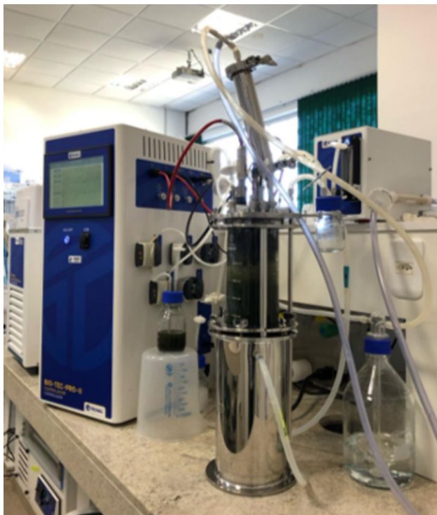
Fig. 1 Airlift benchtop bioreactor, model Bio-Tec-Pro-II (Tecnal, Brazil)
