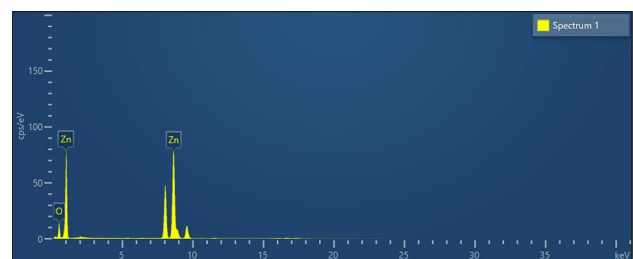
Fig. 7 EDX spectrum of ZnONPs
