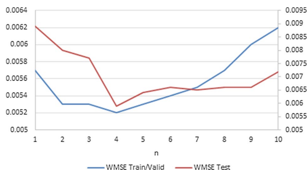
Fig. 3 Weighted mean squared error (WMSE) for the train/valid and test partitions of the Doehlert data set as function of aggregation number, n , i.e., number of best hybrid models to aggregate
