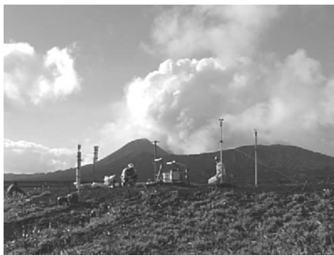
Fig. 2 Photograph from the south of the measurement station on Ambrym Volcano, showing the transmitting antenna and several meteorological sensors
