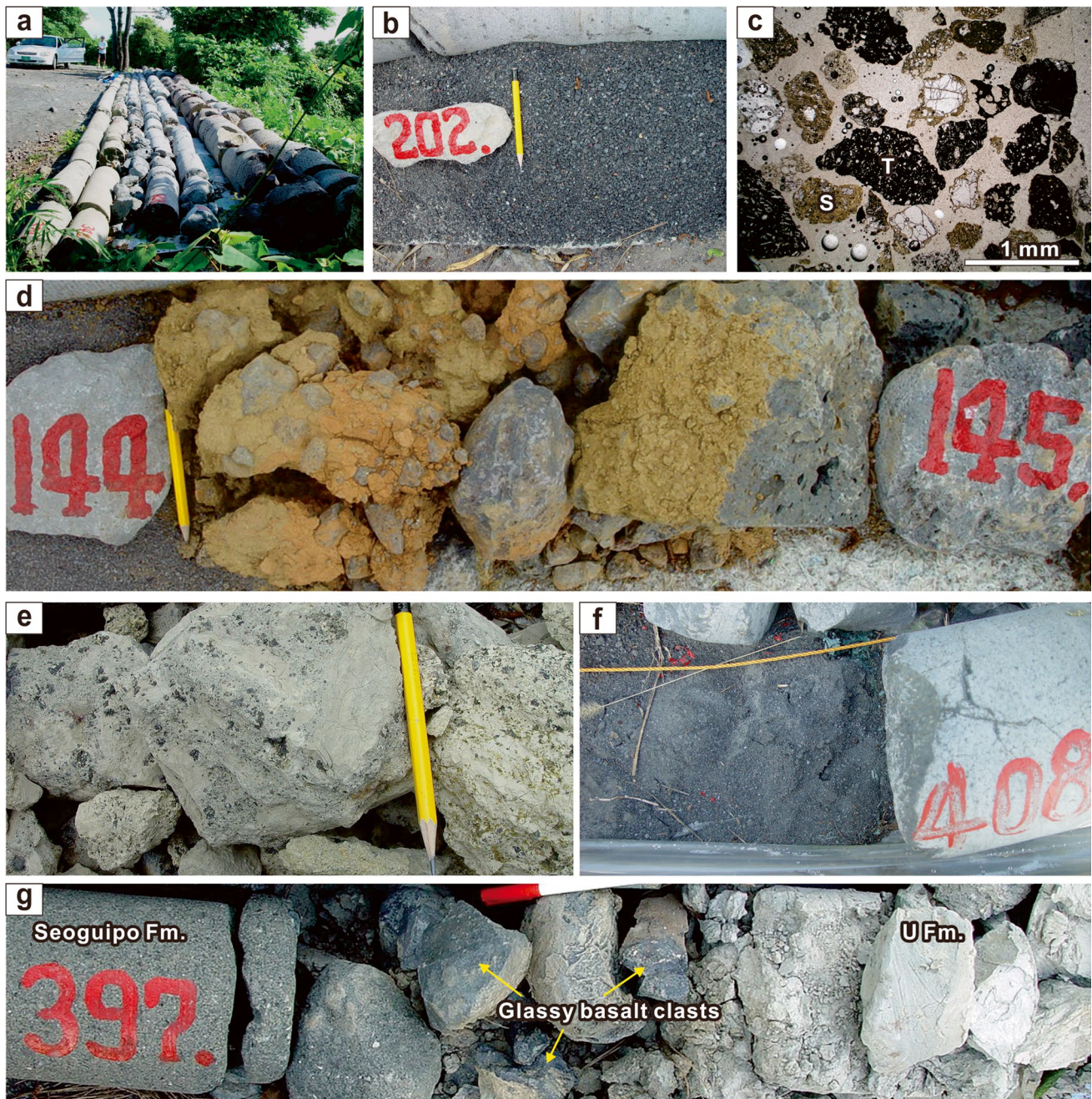
Fig. 4 General features of the Hankyung and Jongdal cores. a A view of the Hankyung core. b Black basaltic sand and granule (hyaloclastite) (Hankyung core; depth: 202 m). c Thin-section photomicrograph of the hyaloclastite shown in b , composed of non-vesicular and angular sideromelane (S) and tachylite (T) particles. d Reddish brown and poorly sorted mud containing basalt clasts, interpreted to be a paleosol layer intercalated between two lava flow units (Hankyung core; depth: 144–145 m). e Massive mudstone with deformed
