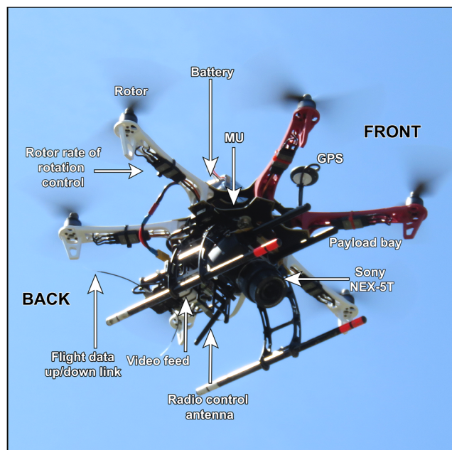
Fig. 2 The platform and sensor system used during the survey. MU stands for management unit
