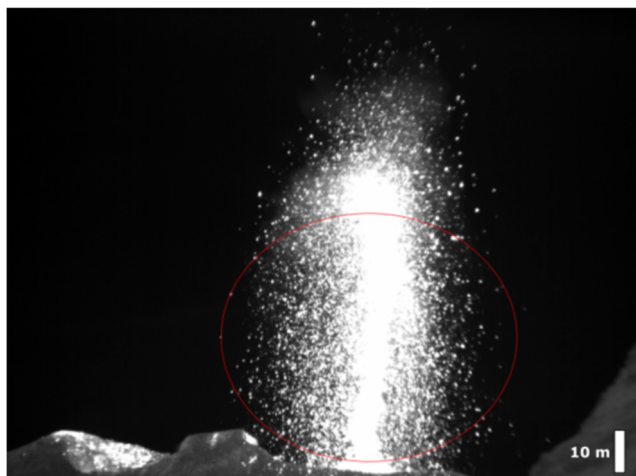
Fig. 4 Example of the simulation of a radiometer field of view in thermal imagery (thermal image of North-East crater at Stromboli taken on 18 May 2014)
