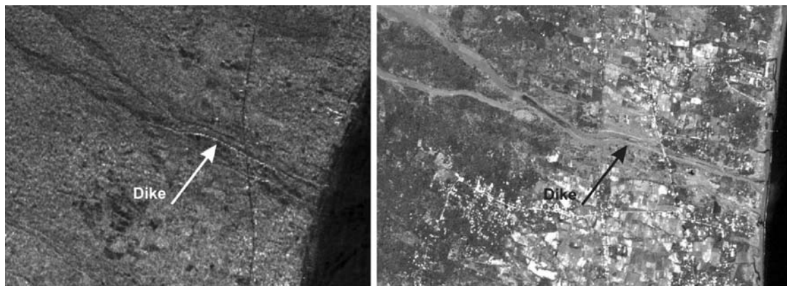
Fig. 3 Concrete dikes appear as light-colored linear features on both radar (a) and optical (b) images
