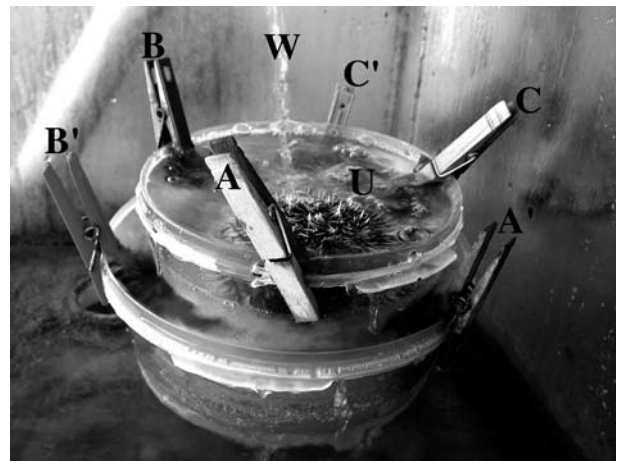
Fig. 1 Design for multiple choice feeding experiments showing experimental chamber (food types, A–C, with urchin) nested within the control chamber (food types, A'–C', without urchin). A, A' Galaxaura oblongata , B, B' Dictyota cervicornis , C, C' Thalassia testudinum , U Tripneustes ventricosus , W sea water
