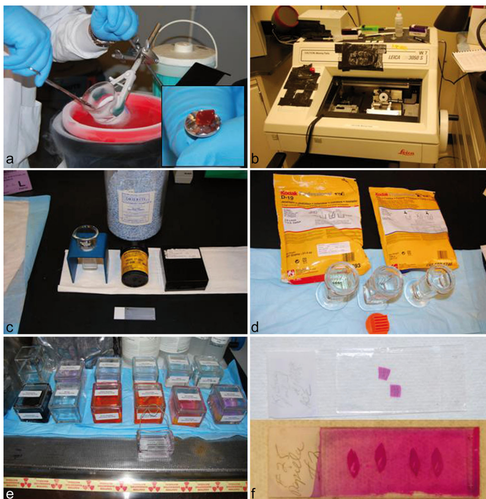
Fig. 2 A pictorial summary of the methods used for MARG. a The snap-freezing apparatus and inset the fresh tissue sample on a cryostat sample holder for mounting and freezing. b A Leica CM3050 Cryostat for cryosectioning of sample and collection onto slides pre-coated with emulsion (note sections must be collected onto glass slides that have been pre-coated with photo-emulsion while under darkroom conditions, thus all equipment lights have been covered with black tape). c Dip Miser slide coating cup (Electron Microscopy Sciences), Kodak emulsion, black slide exposure box, Drierite desiccant and a coated slide. Slides are dipped into liquid emulsion heated in the Dip Miser and allowed to
