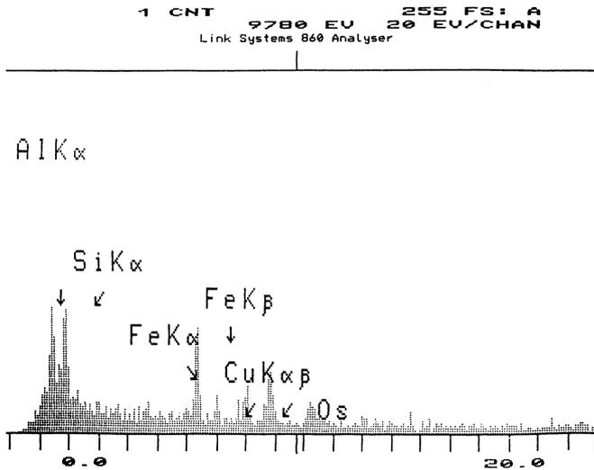
**Fig. 12** *P. multae*: an X-ray energy spectrum from the analysis of an electron-dense granule in a pigmented cell. The K $\alpha$  and K $\beta$  peaks for iron (Fe) represent the principal constituent element. The copper (Cu) and silicon (Si) peaks represent extraneous elements derived from the microscope column and the embedding medium, respectively
