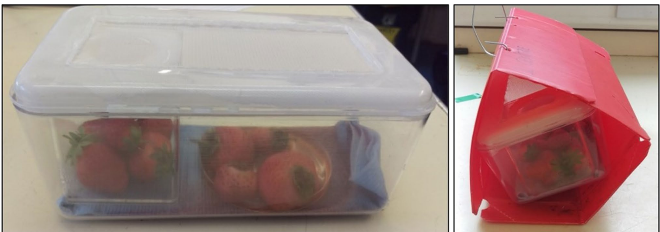
Fig. 1 Left: fruit-baited sentinel trap box containing inoculated strawberries within a Petri dish (right) and non-inoculated fresh fruit in a ventilated small Perspex box (left). Right: sentinel fruit box inserted into red delta trap for deployment in the field
