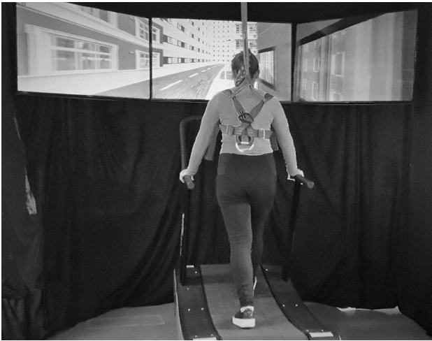
Fig. 1 Experimental setup of VR city. A participant stands on the treadmill and faces VR City
