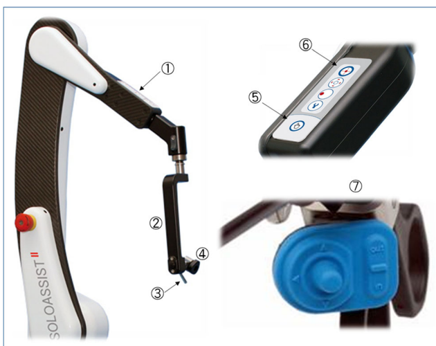
Fig. 1 Soloassist II® camera control system. ① Control panel. ② Universal joint. ③ Probe check. ④ Camera clamp. ⑤ Unlock button. ⑥ Trocar point. ⑦ Joystick
