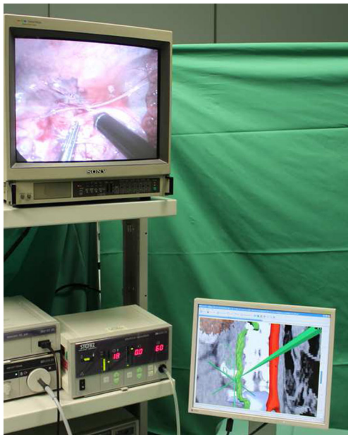
Fig. 2 Navigation system for laparoscopic rectal surgery in a porcine model. A primary screen shows the laparoscopic video and a secondary screen visualizes the aorta and the ureter in relation to the instruments
