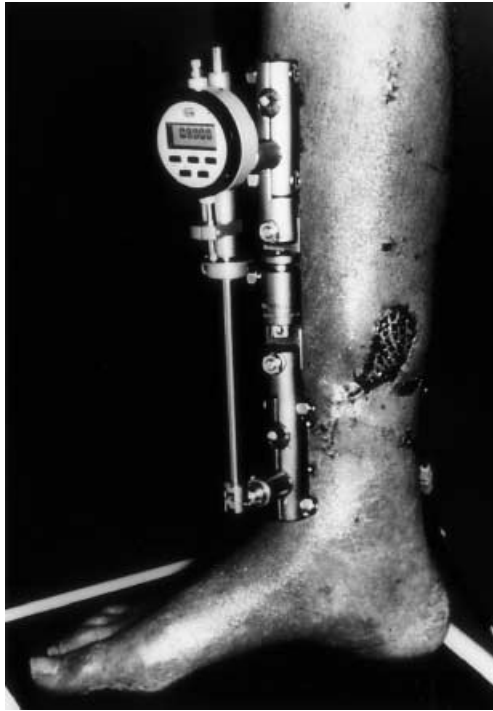
Fig. 1 Axial loading of a tibial fracture stabilized by an Unifix external fixator instrumented with a Fraktometer FM 100 for measurement of fixator deformation (indirect measurement of fracture callus stiffness)
