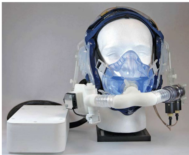
Fig. 5 Prototype of the NASA—PUMA metabolic system modified with permission from NASA (National Aeronautics and Space Administration 2017)
