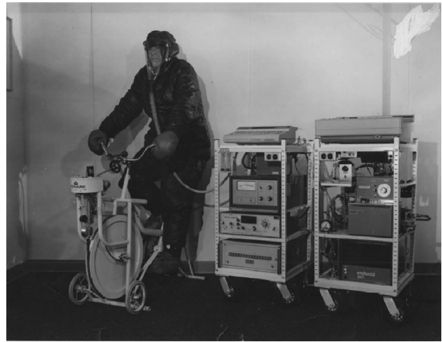
Fig. 5 Suit calorimeter worn by a participant exercising on a cycle ergometer. The insulating garments cover the water-cooled suit which connects to the hardware for controlling water temperature, located on the equipment cart to the right side of the participant. An automated metabolic unit is used to measure gas exchanges. Image is reproduced with permission from the Paul Webb Collection, Wright University Special Collections, and Archives
