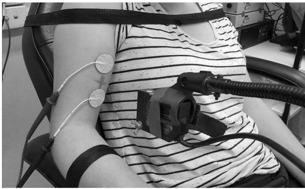
Fig. 1 Demonstration of MMG protocol. After determining 50 % total length of the biceps brachii for MMG laser positioning, proximal and distal stimulator electrodes (TENS pads) were attached 25 mm apart. Upper limb was kept in 90° elbow flexion in a supinated position. Straps were secured around the arm and upper thoracic region to prevent excessive movement during stimulation. MMG mechanomyography
