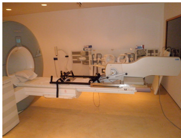
Fig. 1 MRI compatible braked cycle ergometer (Lode BV Groningen) mounted onto a whole body MRI system (Siemens Avanto 1.5 T; Siemens Medical Solutions; Erlangen Germany). Handlebars reduce upper body movement, straps around thighs increase stability and prevent hip movement
