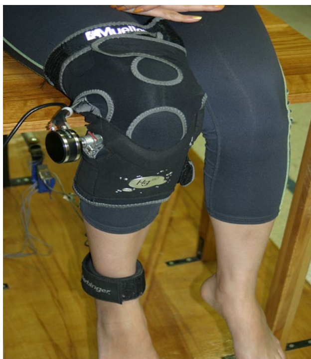
Fig. 2 Experimental setup for measuring FFK and KFEH of the knee. The subject was positioned sitting with the hip and knee flexed to 90°
