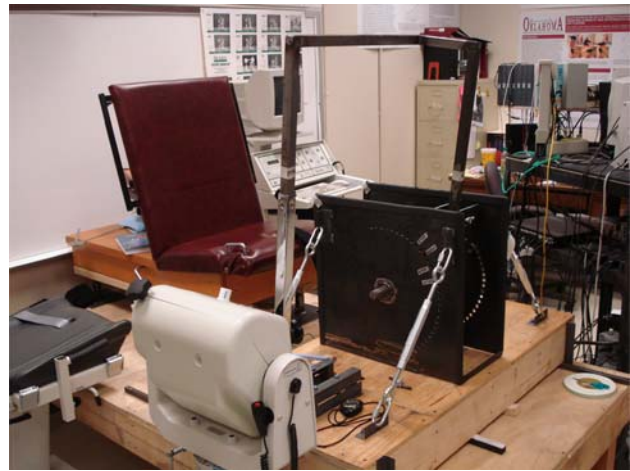
Fig. 1 Custom-built apparatus equipped with a load cell designed for passive stretching and evoked-twitch assessments
