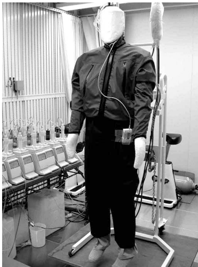
Fig. 1 The newly developed sweating thermal manikin made by Kyoto Electronics Manufacturing, Japan ( KEM manikin ). The body consists of 17 segments, thus, it can realise any desired posture. A wide range of sweating rate can be independently controlled in each segment from 0 \text{ g m}^{-2} \text{ h}^{-1} to 1,500 \text{ g m}^{-2} \text{ h}^{-1}
