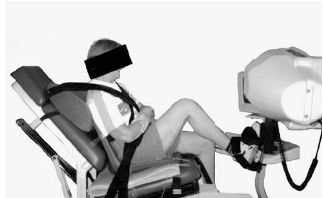
Fig. 1 Dynamometer adopted to perform both isometric and power measures during the leg-press of the dominant limb. The seat was modified in order to have a firm support placed behind the buttock. The trunk was fastened by three belts and each subject's leg was positioned so that a starting angle of 90° at the hip, knee and ankle joint was obtained
