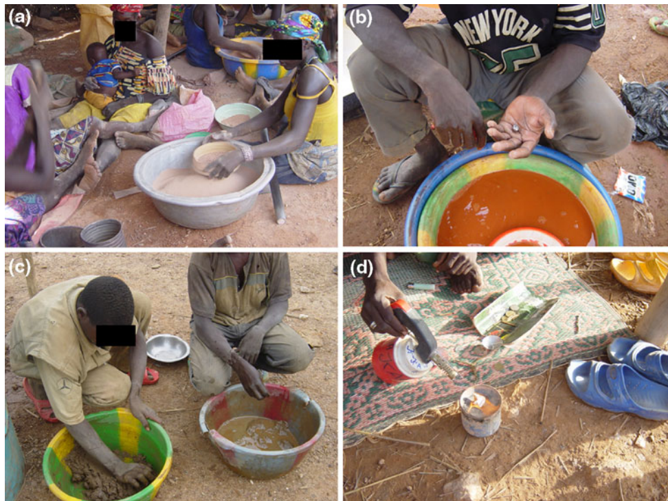
Fig. 1 Different steps during the mining process using mercury, on a small-scale gold mine site in Burkina Faso, with (a) ore crushing,
