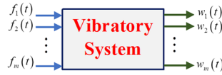
Fig. 1 Schematic view of an MDOF system, where f_i(\omega) and w_i(\omega) are the i th input and output, respectively
