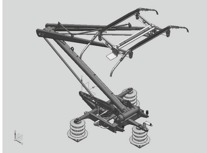
Fig. 1 CAD model of the high-speed railway CX pantograph
