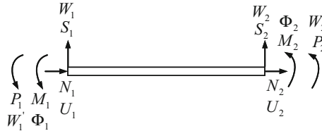
Fig. 3 Boundary conditions for generalized displacements and generalized forces of laminated beam
