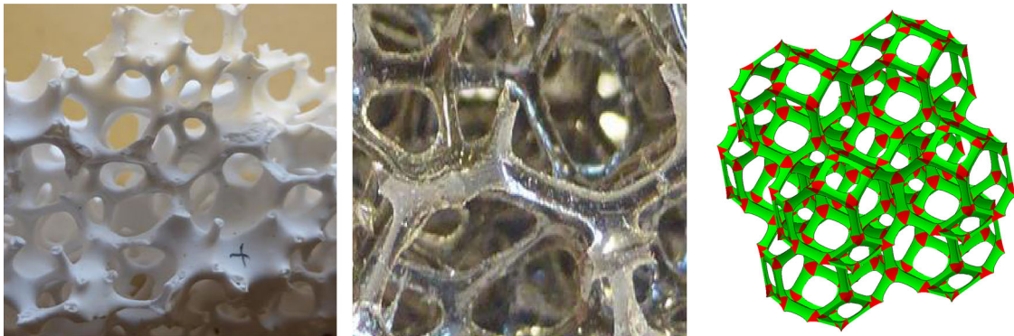
Fig. 1 Broken ceramic foam, polyurethane foam, surface evolver [7] model of a wet Kelvin foam
