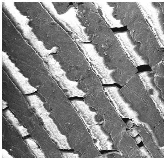
Fig. 1 Transverse cracks in ceramic layer of metal/ceramic composite with lamellar microstructure
