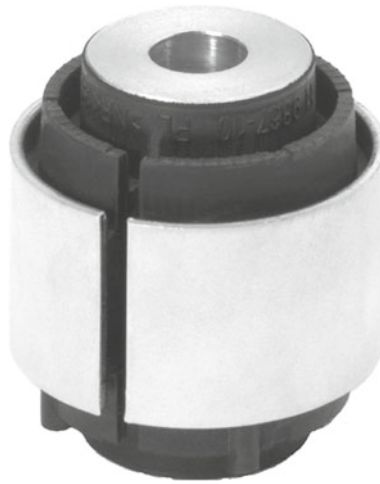
Fig. 2 Example of a bushing used in automotive vehicles (Vorwerk Automotive GmbH & Co KG)
