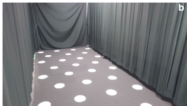
Fig. 1 Mobility test. a. Pattern diagram of the mobility test course. On a black carpet with dimensions of 6 m and 2.2 m, white cloth circles with a radius of 10 cm are placed as obstacles at 40 cm intervals. b. Actual picture of the mobility test course
