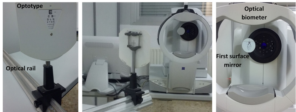
Fig. 2 Some pictures of the experimental setup, including the optical rail used to place the optotype at the required distance depending on the vergence tested and the first surface mirror attached to the optical biometer
