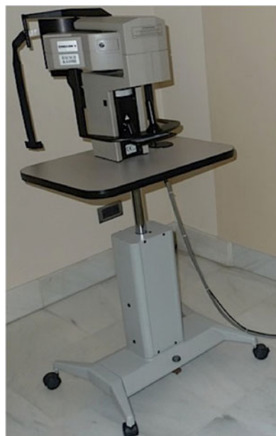
Fig. 1 Photograph of the Orbscan II used in this study ( left ), with a scheme ( right ) marking pupil centre and Placido Disc centres used to calculate angle Kappa
