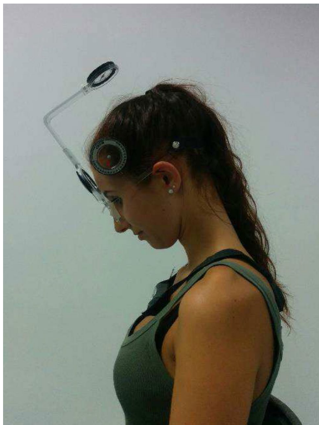
Fig. 1 Cervical range of motion (CROM) validated instrument used to precisely assess the severity of dystonia by measuring cervical rotation, lateral flexion, flexion and extension degrees and to detect the effect of sensory trick on the head position
