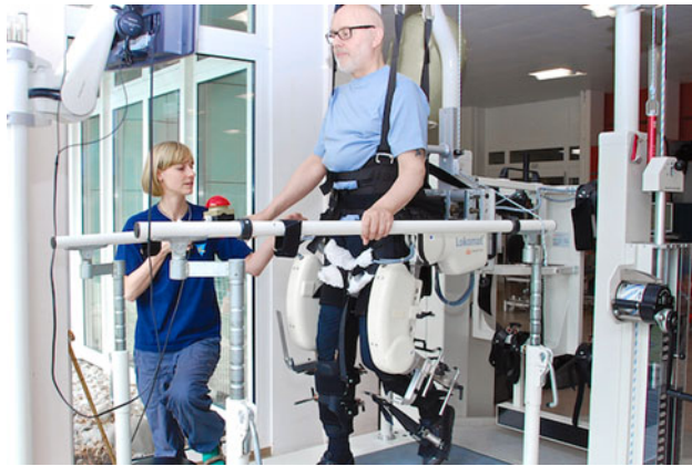
Fig. 4 A stroke patient using a “gait machine” in robotic-assisted gait training (RAGT) under supervision of a physiotherapist
