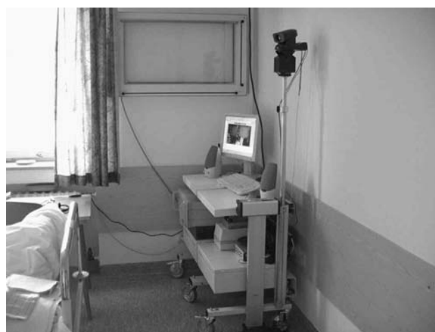
Fig. 1 Telemedicine infrastructure at the local hospital. Remote controlled camera connected to the video server and PC. An X-ray viewer is located in a 90° angle to provide optimal view for CT scans
